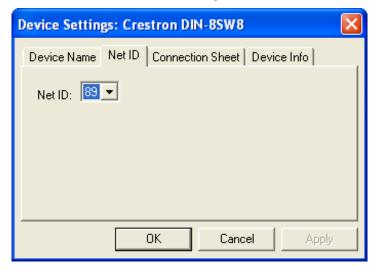
• The ID code specified in the SIMPL Windows program must match the Net ID of each unit. Refer to "Identity Code" which starts on page 10.
